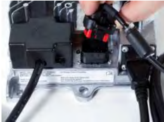
Figure 42: Inserting the AMPSEAL Plug
