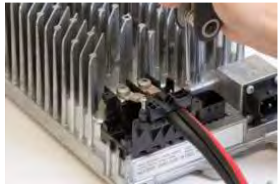
Figure 38: Using the Cable Clamp
