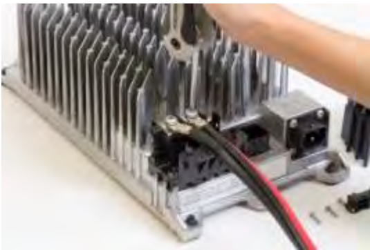
Figure 37: Secure DC Wires
